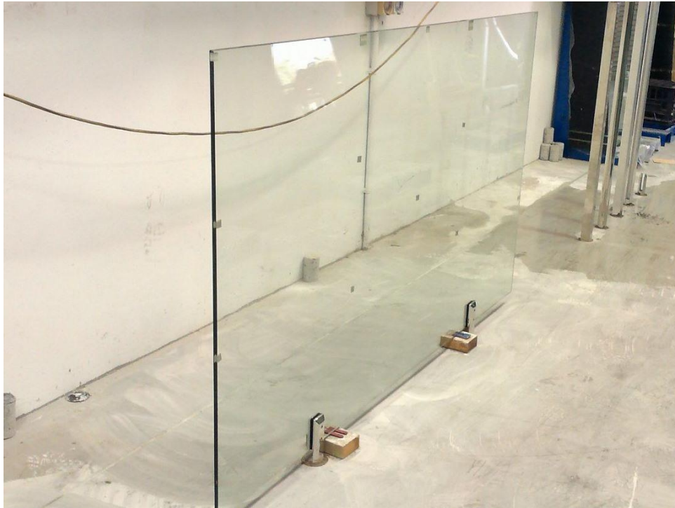
The frameless glass panel as installed.
